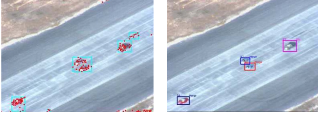
(a) Outlier feature points and initial cluster of objects (b) Final list of objects after data association step
