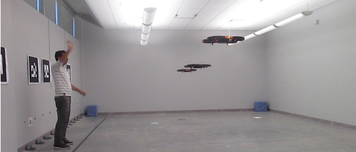
Figure 3.1: An uninstrumented person creates and commands a team of three UAVs using face-engagement and hand gestures
