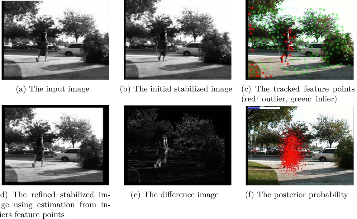
Figure 2.12: The different steps of Jung and Sukhatme [80]’s pipeline for detecting moving objects from a moving platform (© 2009, Springer Science & Business Media BV)
