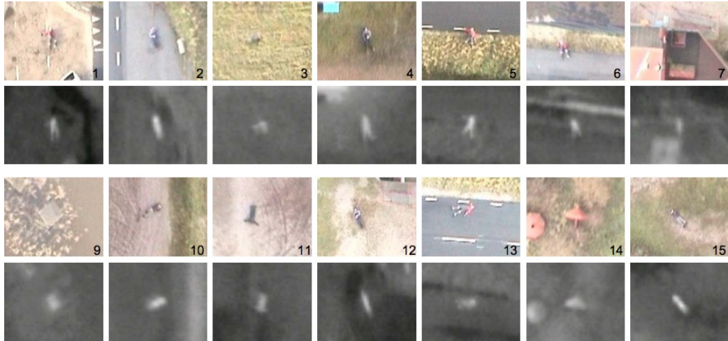
(a) Sample images from Doherty and Rudol [42, 152]’s experiments. The odd rows show RGB images, while even rows show corresponding thermal images.
