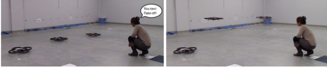
Figure 2.22: Multi-modal interaction system of Pourmehr et al. [142] for Human-mutli UAV interaction (© 2013, IEEE)
