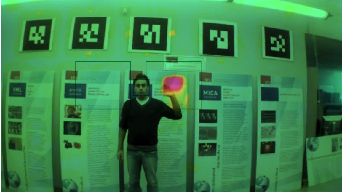
Figure 3.3: Face detection is used to locate the user, and to select the currently focused robot. Hand gestures change the state of the focused robot. This image is from the flying robot’s point of view. The gesture detection regions are marked by a rectangle. (The stabilized optical flow magnitude’s heat map is blended into the image.)
