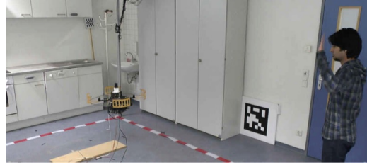
(b) The UAV follows a human and responds to his hand gestures (Naseer et al. [125]) (© 2013, IEEE)
