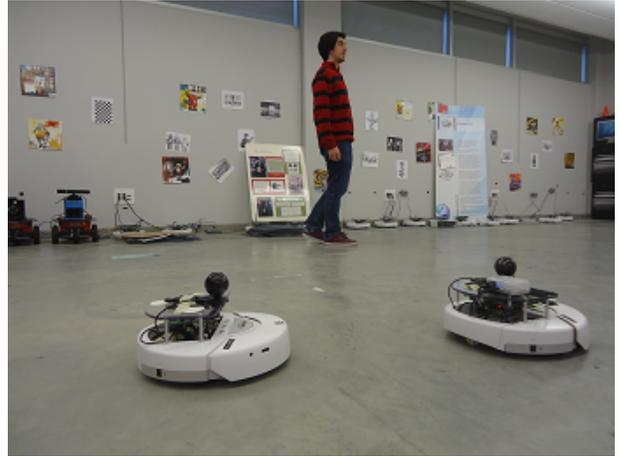
Fig. 1: Two robots following and orbiting a human using CoSLAM as the only sensor.
