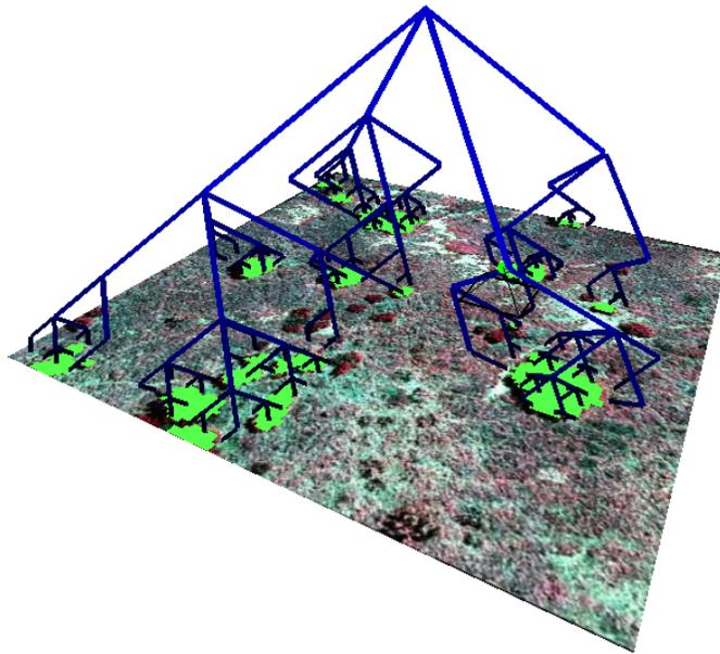
Fig. 1: Simulated environment for area coverage with UAV. Interesting regions are colored green. The lines show the interesting branches of the coverage tree.
