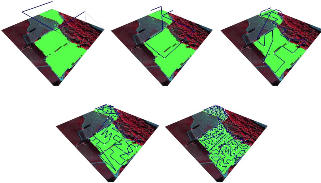
Fig. 7: Sample real environments are simulated in the second experiment. These figures show the coverage plan (generated by TSP 2-approximation) for each level of the tree in the BF strategy. At the first level with no prior interestingness information, coarse lawn mower pattern is performed. Light green (light grey) pixels are interesting.
