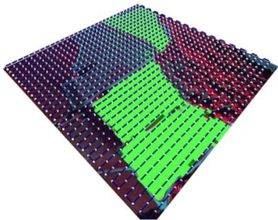
Fig. 6: Lawnmower-like pattern is used as the baseline approach. The area is covered with a uniform resolution.
