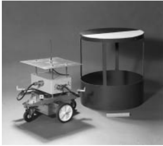
Figure 2: Finished Rover the Robot Sheepdog , with cover removed.
