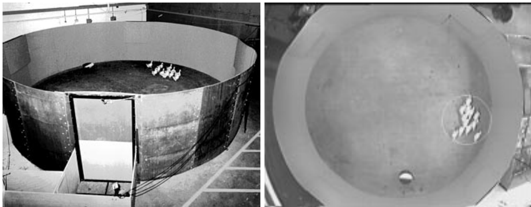
Fig. 3. The experimental arena (left) and view from overhead camera (right). Note the positions of the robot and flock overlaid by the tracker
