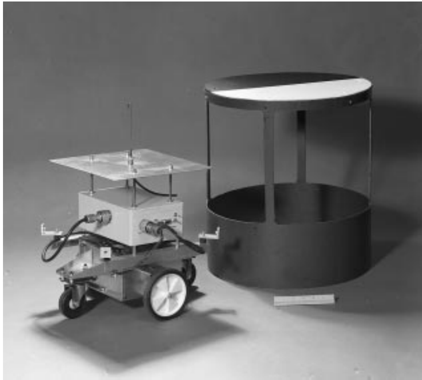
Figure 3.7: Rover #3: final chassis with radio base-plate and original tall cover (removed for clarity).
