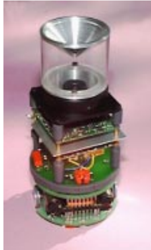
Figure 6.20: A Khepera robot fitted with a small CCD camera and conical mirror. This arrangement provides a 360^\circ view in the image projected onto the camera.
