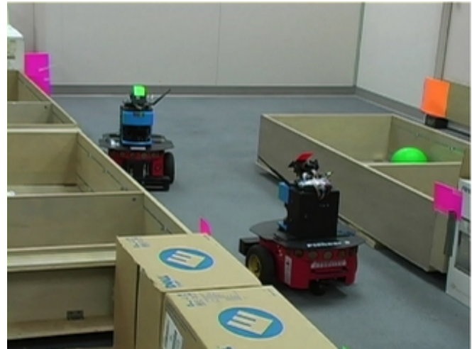
Fig. 1. Spatial-Interference: two robots block each others’ way in a narrow corridor [11].
