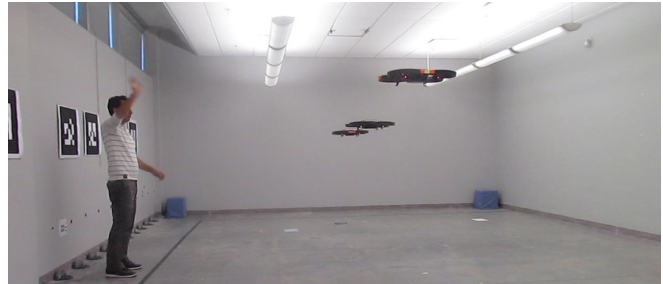
Fig. 1. An uninstrumented person creates and commands teams of UAVs using face-engagement and hand gestures
