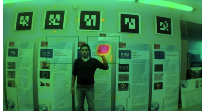
Fig. 3. Face detection is used to locate the user, and to select the currently focused robot. Hand gestures change the state of the focused robot. This image is from the flying robot’s point of view. The gesture detection regions are marked by a rectangle. (The stabilized optical flow magnitude’s heat map is blended into the image.)
