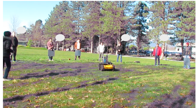
Fig. 6: Setup of experiment IV-B: Eight human participants are positioned in a semi-circle with radius 7 meter around the robot. Individuals create specific sensor stimuli by shouting, covering their legs or standing outside the field of view of a particular sensor.
