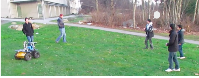
Fig. 2: Real-world setting (university campus) for experiment IV-A with five uninstrumented users at arbitrary poses. One person, chosen at random, tries to get the robot’s attention, and the robot reliably approaches him.
