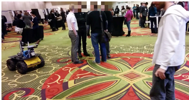
Fig. 1: The mobile robot is able to robustly track people and attend the most engaging person to deliver its service, despite the noisy and crowded environment. (live demonstration at HRI’14 )
