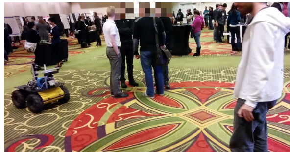
Fig. 1: A live demonstration at HRI’15. The mobile robot is able to robustly track people and approach the most engaging person, despite the noisy and crowded environment.
