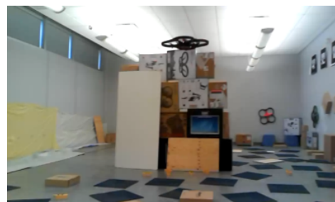
(a) Experimental arena. With no initial map, and using only mono-SLAM, the MAV must navigate around obstacles to reach a goal point. The left-hand part of the room has few visual features and is unsafe for navigation.
